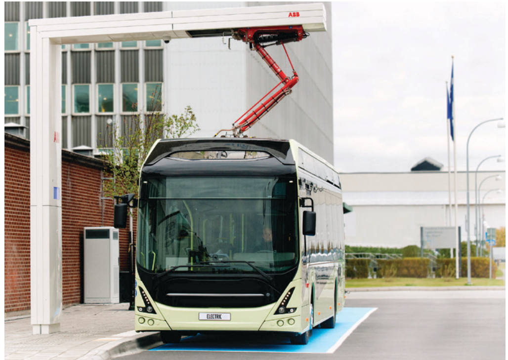
Figure 7: Pantograph charging (Volvo Buses 2016)
